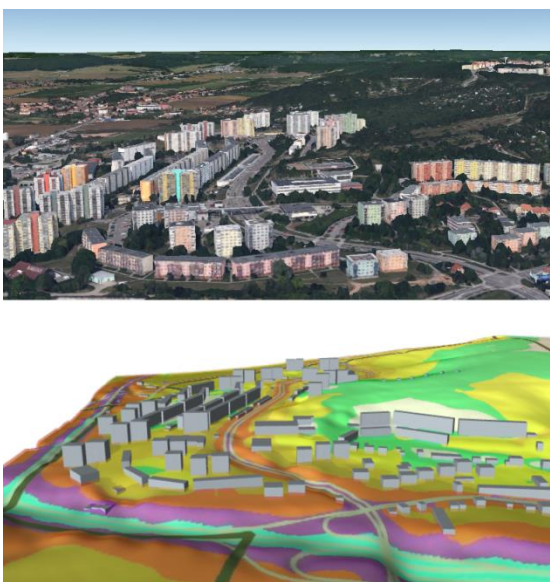
Fig. 3. Photorealistic visualization from Google Earth and abstract visualization of 3D noise map. Area of city district
